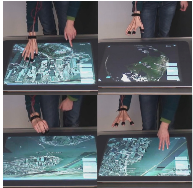
Figure 4: Multi-touch scaling using two fingers (top left), HAND_SPREAD to zoom (top right), HAND_GRAB gesture to translate the map (bottom left), and combination of a touch HOLD and point HAND_SPREAD gesture to tilt the map.
