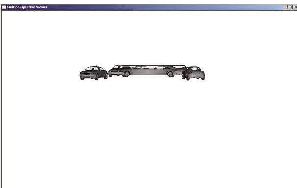
Figure 7: Multiperspective View of the three-dimensional scene. The users' head is located above the middle of the display ( y -coordinate), in the horizontal centre ( x -coordinate). The distance to the display ( z -coordinate) is larger than in Figure 5. The interface renders a multiperspective view on in the middle and a perspective view on the left and on the right side.
