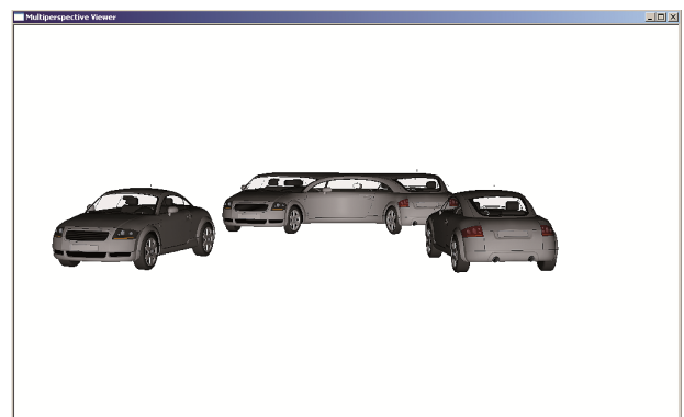
Figure 5: Multiperspective view of the three-dimensional scene. The user is located in the centre (x- and y-coordinate) in front of the display. The interface renders a multiperspective view in the central area and a perspective view in the outer regions
